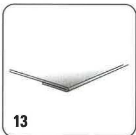
13 FOLD AT FRONT OF SHELF reinforces the shelf and protects specimen folders.
