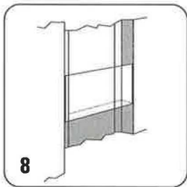
8 FUMIGANT COMPARTMENTS are built into the inside of the door.
